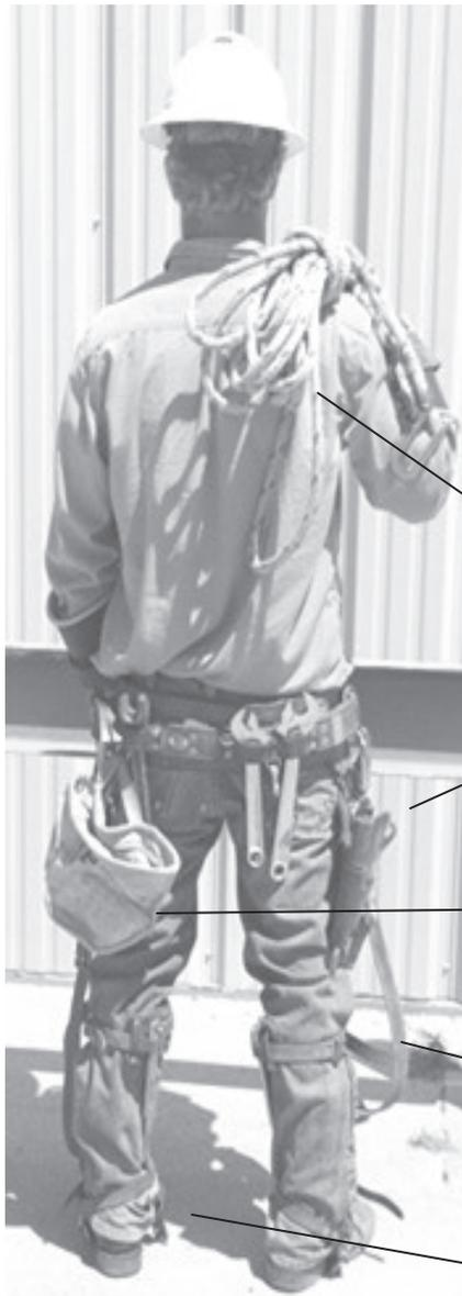
**Fall Protection Belt** is the primary OSHA belt mandatory by April 2015. With its cinch lock, this belt cinches over the top of an object to be the main fall protection, securing a lineman at all times.
